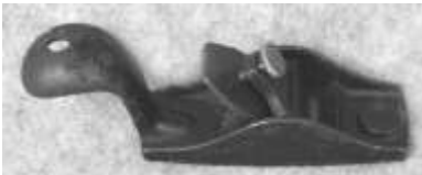
Figure 656. Stanley No. 100 tailed block plane. Cast iron, japanned finish, steel blade. CLT. 81212LTC10.
