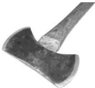
Figure 194. Double bit ax. Cast steel, wood (hickory). Plumb. DTM. 12813T2.
