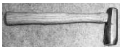
Figure 50. Doghead saw hammer. Steel, wooden handle. Henry Disston & Sons. DTM. 102512T7.
