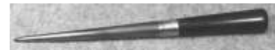
Figure 536. Marlin spike. Cast steel, brass ferrule, hardwood handle (ebony?), ivory butt. CLT. 81212T1.
