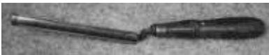
Figure 425. Crane neck gouge. Cast steel, brass ferrule, wooden handle. Buck Brothers. DTM. 42904T4A.
