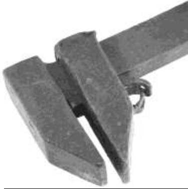
Figure 4. Wedge adjusted wrench. A simple machine that can be dated in its origin to the early Iron Age – 1200 BC. DTM. 21812T21.
