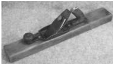
Figure 277. Wood bottom transitional jointer plane. Wood (beech) body and handles, cast iron fittings. Birmingham Plane Co. CLT. 72312LTC4.
