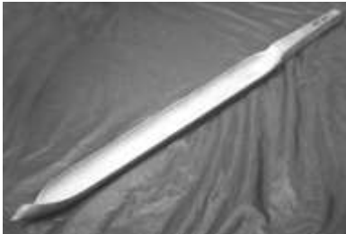
Figure 248. Pipe or pump auger bit. Forged iron. DTM. TBA1004.
