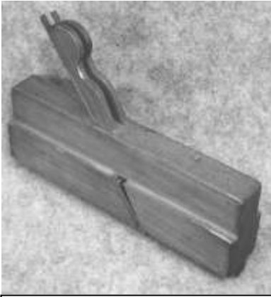
Figure 270. Double sash plane. Wood (beech), steel blade. DTM. 31808SLP5.
