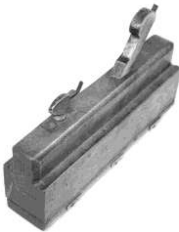
Figure 283. Moving filletster plane. Wood (beech), steel. James Clark. CLT. 3713T4.
