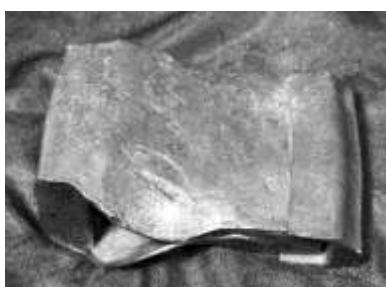
Figure 31. Unfinished ax head with forge-welded edge. Forged iron and steel. DTM. 81411T1.
