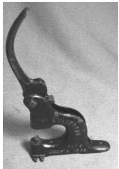
Figure 710. Right: Riveting machine. Malleable cast iron, japanned finish. F.H. Smith Mfg. Co. CLT. 72712LTC9.
