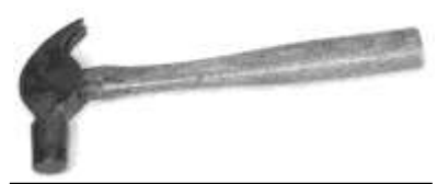
Figure 165. Scotch pattern farriers' hammer. Cast steel, wood (hickory). DTM. 12613T2.
