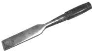
Figure 302. Timber framing chisel. Forged iron, cast steel, wood. Buck Brothers. DTM. 31908T20.
