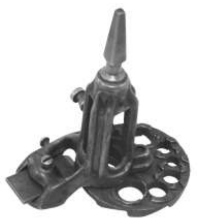
Figure 349. Adjustable hollow auger bit. Malleable cast iron, steel. E.C. Stearns. DTM. 101312T23.
