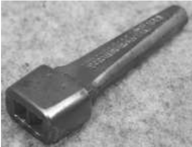
Figure 404. Saw swage. Drop-forged steel. Simonds. DTM. 102503T4.
