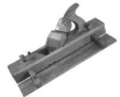
Figure 275. Panel raising plane with adjustable fence. Wood (beech), steel blade. James Cam. DTM. TCD1003.
