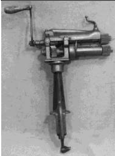
Figure 131. Bench roller with clamp and crankshaft handle. Drop-forged steel. Peck, Stow & Wilcox. CLT. 21812LTC3.
