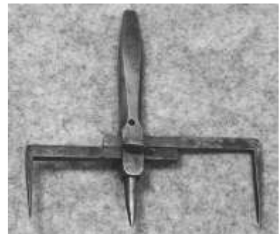
Figure 699. Leather washer cutter. Drop-forged iron and steel. C.S. Osborne & Co. CLT. 42912LTC16.
