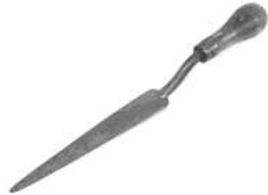
Figure 430. Patternmakers' molding tool. Forged iron, wood (boxwood). DTM. 21013T2.
