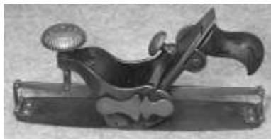
Figure 648. Stanley no. 113 adjustable compass plane. Grey cast iron, tempered alloy steel, steel blade. DTM. 22211T26.
