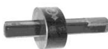
Figure 310. Scratch gauge. Wood (ebony), brass, steel. Robert Fairclough & Co. CLT. 3713T5.
