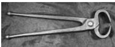
Figure 59. Blacksmiths' end cutters. Drop-forged iron and steel. Heller Brothers. DTM. 31212T1.
