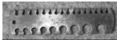
Figure 580. Wire gauge. Steel. The Blodgett Mfg. Co. of Rochester, New York. DTM. 10910T4.
