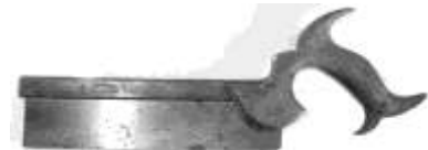
Figure 333. Tenon saw. Tempered alloy steel, brass, and wooden handle R. Groves & Son. DTM. 92911T16.
