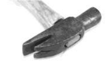
Figure 56. Hammer. Cast steel, wood (hickory). DTM. 31311T7.
