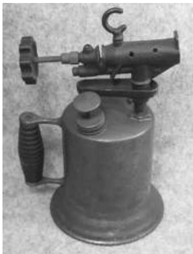
Figure 674. Gasoline blowtorch. Drop-forged steel, brass. CLT. 72712LTC12.
