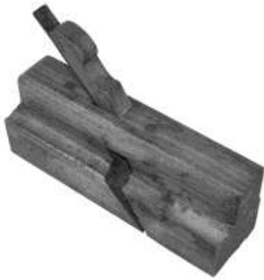
Figure 279. Plane. Wood (beech), steel. Thomas Waterman. DTM. TBW1004.
