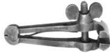
Figure 555. Hand vise. Drop-forged iron or steel. W. & C. Wynn. DTM. 121112T6.
