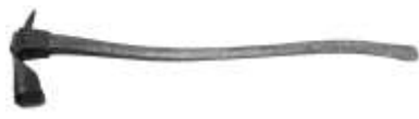
Figure 363. Gutter adz. Forged steel and iron, wooden handle. Jim Sheffield. DTM. 121112T2.
