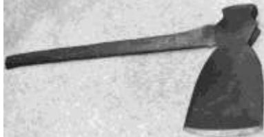
Figure 216. Yankee pattern mast ax. Cast steel, wood. DTM. 102612T2.
