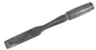
Figure 155. Socket framing chisel. Steel with a forge-welded edge, wood (hickory), iron ferrule. Underhill Edge Tool Co. DTM. 32707T1.
