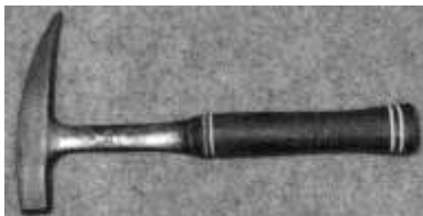
Figure 697. Rock hammer. Drop-forged steel, compressed leather discs. Estwing. DTM. 101312T29.
