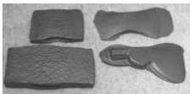
Figure 546. Ax head castings. Cast steel. DTM. 102612T16.
