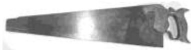
Figure 411. Hand saw. Spring steel, wood (beech). R. Groves & Sons, Sheffield. DTM. 2213T2.
