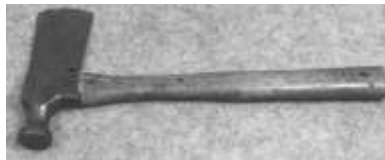
Figure 321. Shingle hatchet. Drop-forged steel, wooden handle. C.A. Williams & Co. DTM. 43006T9.
