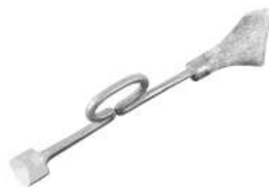
Figure 140. Farriers' buttress (hoof paring tool). Forged malleable iron, wooden handle. DTM. 61612T4.
