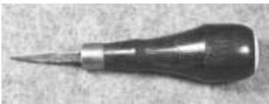
Figure 534. Bodkin. Cast steel, brass ferrule, wood handle (mahogany), ivory inset. CLT. 81212LTC4.
