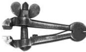
Figure 107. Hand vise. Forged iron or steel. G. Kipp. DTM. TCR1302.
