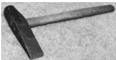
Figure 62. Hot set hammer. Cast steel, wood (hickory). Vulcan. DTM. 101312T6.
