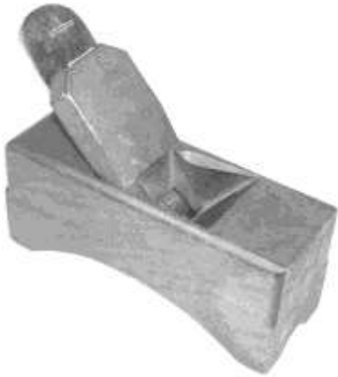
Figure 412. Wheelwright's wooden compass plane. Levi Tinkham. Beech wood, steel. DTM. 51213T1.
