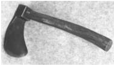
Figure 243. Gutter hand adz. Forged steel, wood (hickory). DTM. 101312T16.
