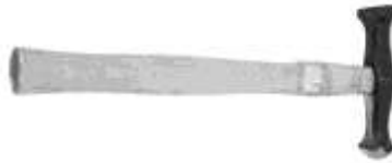
Figure 181. Silversmiths' hammer. Drop-forged steel, wood (hickory). DTM. 121412T7.
