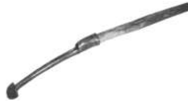
Figure 202. Spud. Malleable iron and steel, wood. DTM. 31808PC6.
