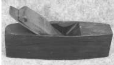
Figure 271. Coffin plane. Rosewood and maple with cast steel blade. DTM. 81801T10.
