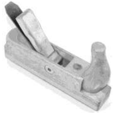
Figure 281. Horned scrub plane. Wood (beech, hornbeam), steel, brass. E.C. Emmerich. CLT. 2713LTC2.
