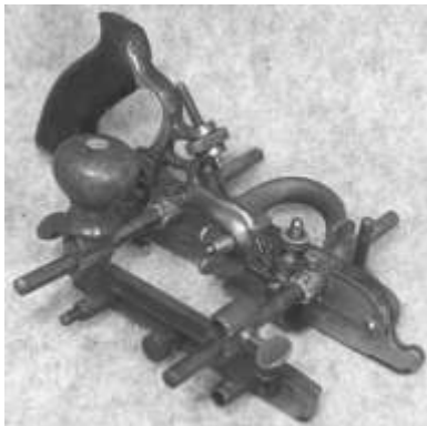
Figure 635. Traut's patent universal combination plane. Grey cast iron, tempered alloy steel, steel blades, brass nuts, with a wooden handle. Stanley. DTM. 22211T29.
