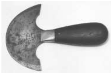
Figure 450. Head knife. Drop-forged steel, brass, wooden (rosewood) handle, leather sheath. C. S. Osborne. CLT. 10112LTC3.
