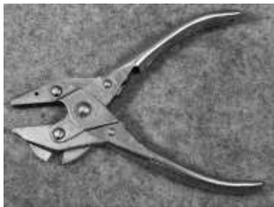
Figure 669. Wire cutting pliers. Nickel-plated drop-forged steel. Sargent & Co. CLT. 42912LTC10.
