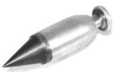
Figure 662. Plumb bob. Turned brass and cast steel. CLT. 3213LTC4.
