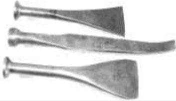
Figure 371. Caulking irons. Cast steel. T Laughlin & Co. CLT. 22813LTC3.
