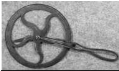
Figure 422. Wagon wheel measuring tool or traveler. Malleable iron, wood. Wiley & Russell Mfg. Co. DTM. 32708T44.
