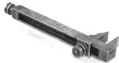
Figure 707. Screw adjusted locking nut wrench. Cast Steel. DTM. 7602T6.
