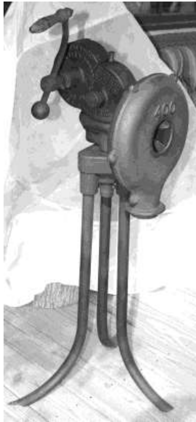
Figure 77. Blacksmiths' blower. Cast iron. Champion. CLT. 62213LTC1.
