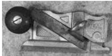
Figure 657. Stanley No. 98 side rabbet plane. Cast iron, wooden (rosewood) knob. CLT. 81212LTC9.
