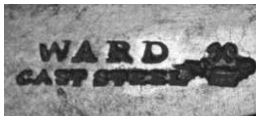
Figure 548. Maker's marks from socket chisels, American on left, English on right. Cast steel. DTM. 102904T12 and 100108T3.
