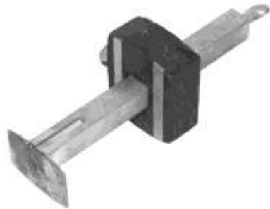
Figure 339. Butt and rabbet gauge. Brass, wood (rosewood). CLT. 122712LTC2.
