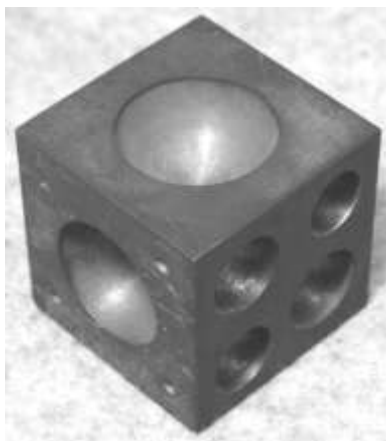
Figure 178. Dapping block, cast steel. DTM. 22512T9.
