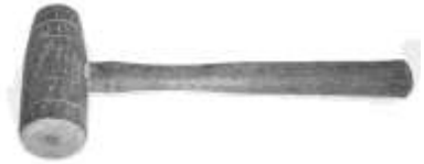
Figure 168. Wooden mallet. Hickory. DTM. 12613T4.
