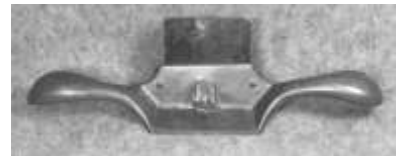
Figure 266. Cast brass scraper. Cast bronze, steel edge. CLT. 81212LTC12.
