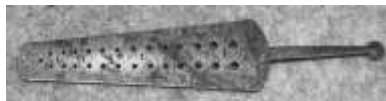
Figure 104. Horologists' and gunsmiths' screw threading plate. Cast steel. Peter S. Stubs. DTM. 42012T2.
