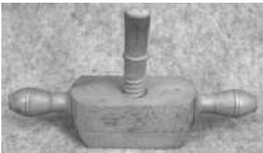
Figure 341. Screw box. Wood and steel. DTM. 112303T1.
