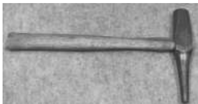
Figure 46. Blacksmiths' round eye punch hammer. Cast steel, wood (hickory). DTM. 101312T21.
