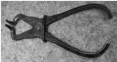
Figure 700. Tire pliers. Drop-forged steel. CLT. 42912LTC12.
