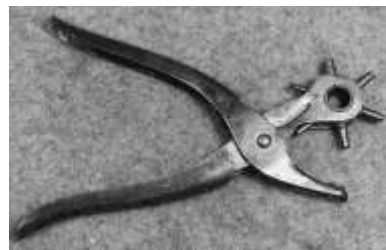
Figure 442. Revolving leather hole punch. Steel. W. Schollhorn of New Haven, Connecticut. CLT. 42812LTC2.
