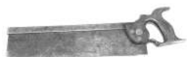
Figure 306. Carpenters' back or tenon saw. Cast steel, wooden handle. I. Colbeck. DTM. 92911T17.
