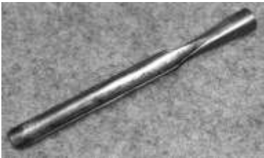
Figure 230. Carpenters' socket gouge. Drop-forged steel. A.W. Crossman. DTM. 32412T5.
