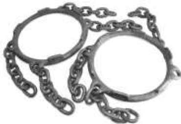
Figure 83. Mast rings. Forged iron/steel. DTM. 12613T3.
