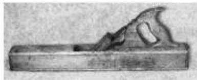
Figure 268. Fore plane. Wood body, Swedish steel cutting edge. Bernard and Oskar Liberg of Rosenfors, Sweden. DTM. 102512T23.
