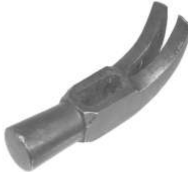
Figure 170. Adz-eye hammer. Cast steel. DTM. 12813T3.
