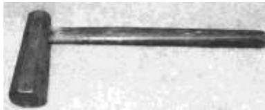
Figure 408. Saw hammer. Steel, wooden handle. Fisher. DTM. 102612T7.
