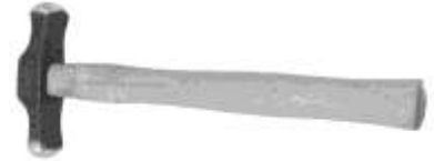
Figure 182. Silversmiths' hammer. Drop-forged steel, wood (hickory). DTM. 121412T6.
