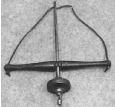
Figure 251. Bow drill. Lathe turned steel, leather, wood. DTM. 8912T1.
