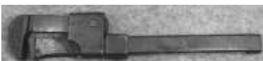
Figure 617. Handle slide adjusting wrench. Malleable iron. H. & E. Wrench Co. (G.E. Hemphill and E.J. Evans). CLT. 32412LTC1.
