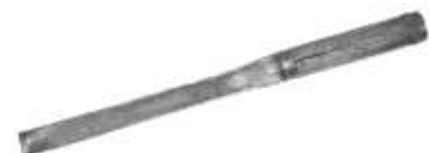
Figure 116. Gouge. Reforged steel file. DTM. 31311T11.
