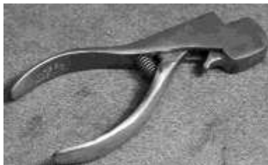
Figure 698. Conductors' railroad punch. Drop-forged steel, nickel-plated finish. McBee. CLT. 72712LTC7.
