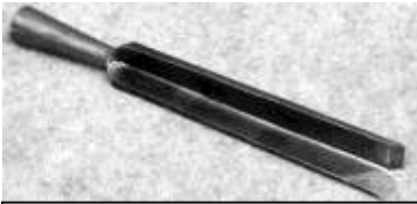
Figure 314. Corner chisel. Cast steel. T.H. Witherby. CLT. 101212LTC3.
