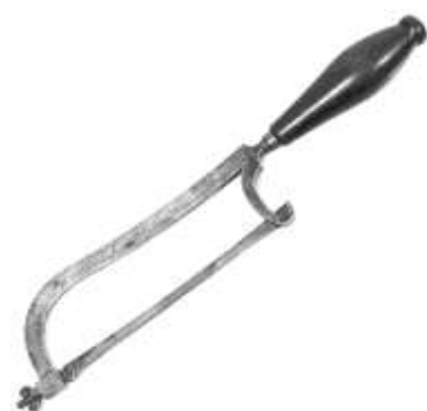
Figure 27. Jewelers' hacksaw. Forged steel, wood (cocobolo), brass. CLT. 31713LTC1.
