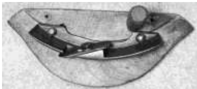
Figure 394. Coopers' croze. Oak body, steel edge. DTM. 102512T22.
