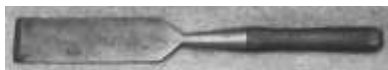
Figure 353. Timber framing chisel. Malleable iron, steel, with forge-welded laminated steel. Gary I. Mix. CLT. 22512LTC13.
