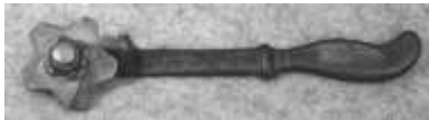
Figure 576. Spring winder. Forged steel, brass, cast iron handle, wooden handle. DTM. TJE1003.
