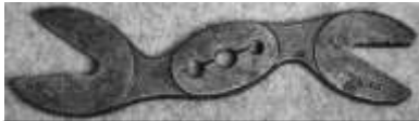
Figure 620. Combination alligator wrench and threader. Cast steel. Hawkeye Wrench Co. of Marshalltown, Iowa. CLT. 7612LTC4.
