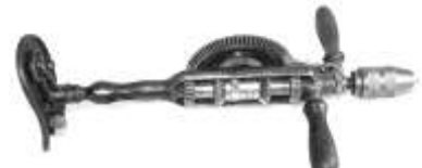
Figure 260. Continuous motion two-speed ratcheting breast drill. Cast iron, steel, wood (rosewood). Millers Falls Co. CLT. 32313LTC6.
