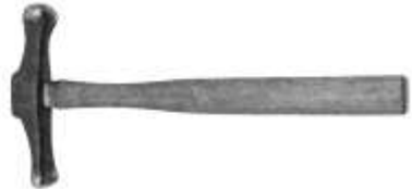
Figure 183. Silversmiths' hammer. Drop-forged steel, wood (hickory). DTM. 121412T10.
