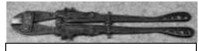
Figure 682. Bolt cutters. Drop-forged steel. John W. Geddes and H.K. Porter of Everett, Massachusetts. CLT. 51012LTC4.
