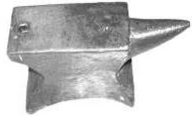
Figure 38. Horned anvil. Iron, forge-welded steel. CLT. 32313LTC1.
