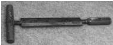
Figure 523. Curriers' fleshing knife. Forged iron and steel, brass ferrule, wood handle. D. Tomlinson. DTM. 62406T2.
