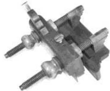
Figure 284. Plow plane. Wood (beech, boxwood), steel. A.B. Semple & Bros. CLT. 32313LTC2.
