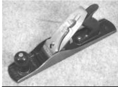
Figure 654. Stanley No. 5 jack plane. Grey cast iron, wood (rosewood), brass knobs, japanned finish. CLT. 7512LTC1.
