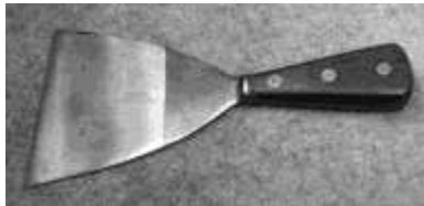
Figure 695. Putty knife and scraper. Drop-forged malleable iron or steel blade, rosewood handle. John Russell & Co. Green River Works, Greenfield, Massachusetts. DTM. 3312T16.
