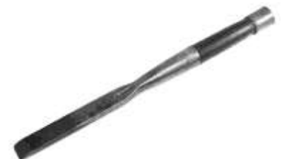
Figure 325. Mortising chisel. Cast steel, forged steel, wood (hickory), brass. William Ash & Co. DTM. 32313LTC5.
