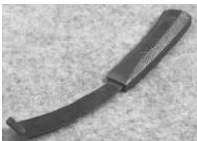
Figure 141. Pope's iron handle farrier knife. Malleable iron handle, steel blade. T.J. Pope. DTM. 32412T6.
