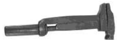
Figure 108. Adjustable wrench. Forged iron. DTM. TBK1001.
