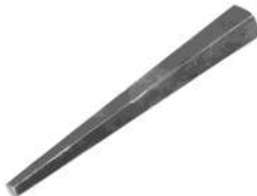
Figure 44. Mandrel. Cast steel. CLT. 22813LTC10.
