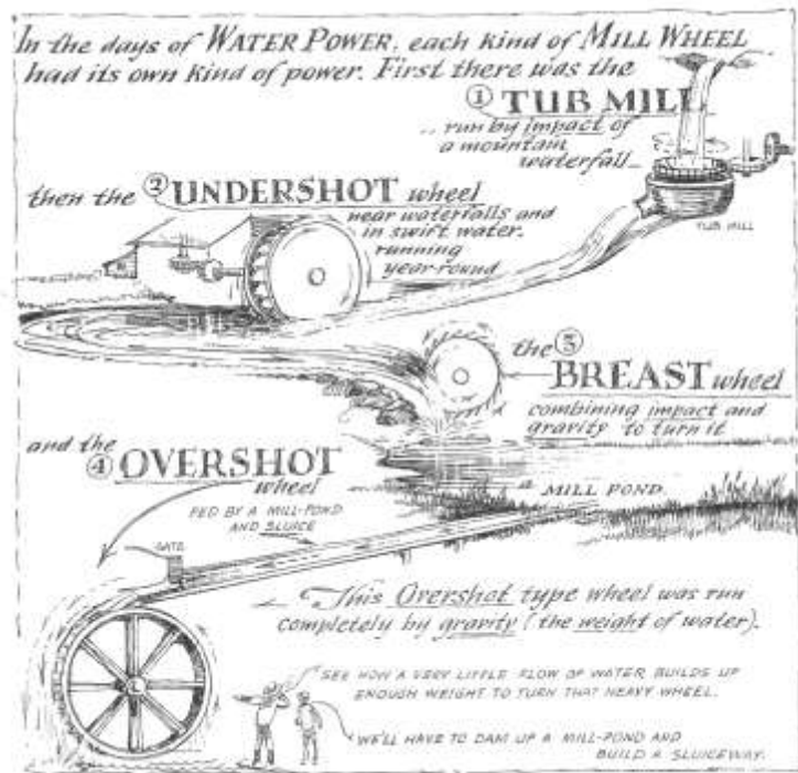
Figure 29. Mill wheels, from Diary of an Early American Boy , Noah Blake 1805. Eric Sloane (2004) Dover Publications.
