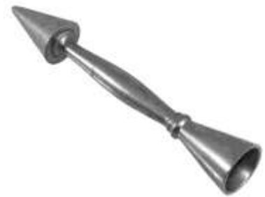
Figure 719. Organ tuning cone. Lathe turned steel. DTM. 12413T1.
