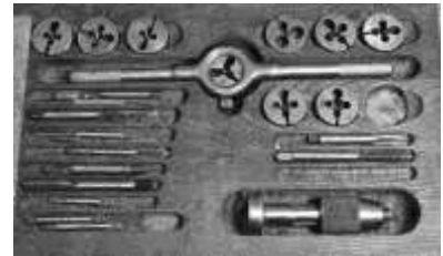
Figure 595. Tap and die set. Drop-forged tempered alloy steel, drop-forged steel bits. CLT. 22512LTC6.
