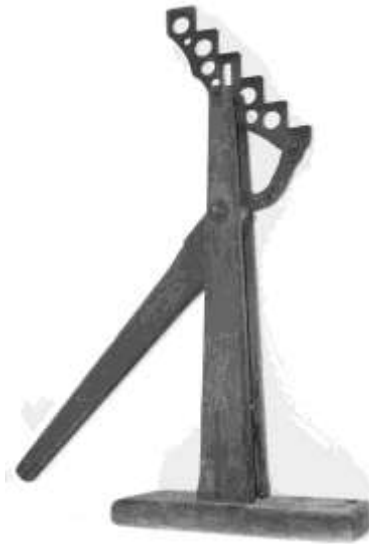
Figure 413. Wagon jack. Cast steel, wood (hickory). DTM. 2713T4.
