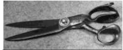
Figure 690. Upholsterers' shears. Cast steel, brass. CLT. 72712LTC8.
