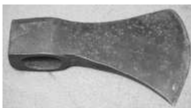
Figure 195. Hewing ax. German or blister steel. DTM. 111006T2.
