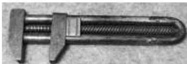
Figure 627. Slide adjusted nut wrench. Drop-forged steel, brass. DTM. 32708T52.
