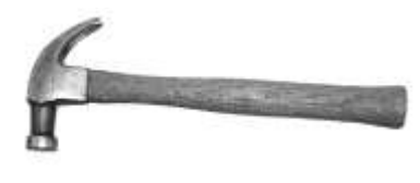
Figure 164. Stanley claw hammer. Cast steel, wood (hickory). Stanley. DTM. 121412T2.
