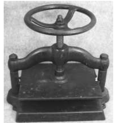
Figure 687. Book press. Cast iron, japanned finish. CLT. 72312LTC1.
