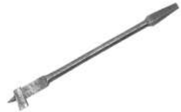
Figure 257. Expansive bit. Drop-forged steel. W. A. Ives Mfg. Co. DTM. 111412T1.
