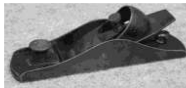
Figure 643. Bailey no. F block plane. Grey cast iron, cast steel blade. Bailey Tool Co., Woonsocket, Rhode Island. DTM. 100400T1.
