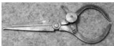
Figure 25. Combination calipers. Cast steel or German steel with brass knob and copper rivet. Peter S. Stubs. DTM. 22411T24.
