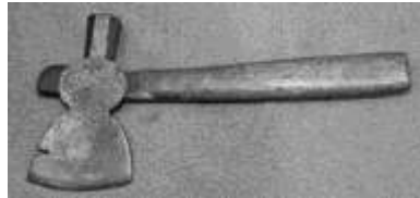
Figure 228. Shingling hatchet. Forged iron and steel, wood. Underhill Edge Tool Co. DTM. TCC3003.
