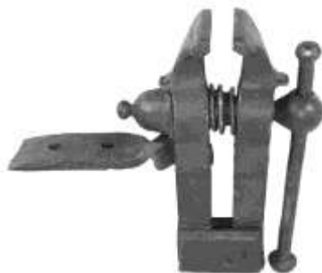
Figure 41. Post vise. Forged iron. DTM. TBF1004.
