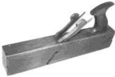
Figure 285. Toted double cutter door plane. Wood (beech), cast steel. Levi Tinkham. DTM. 32313T1.
