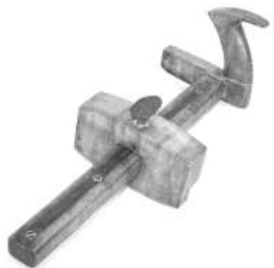
Figure 329. Slitting gauge. Wood, forged iron. DTM. 42801T11.
