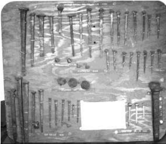
Figure 95. Nail display. Hand-forged and machine cut iron nails, wooden display. DTM. 4512T1.
