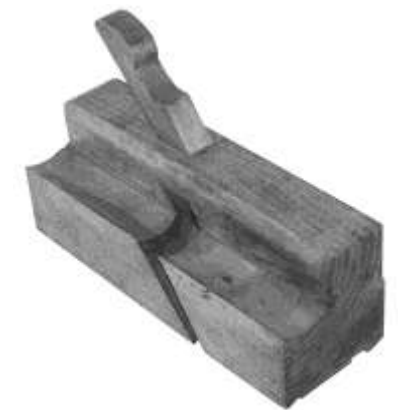
Figure 278. Panel raising plane. Wood (beech). Thomas Waterman. DTM. TBW1003.
