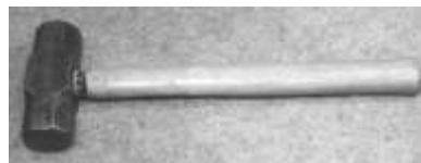
Figure 47. Turning sledge. Drop-forged steel, wood (hickory). CLT. 52612LTC1.
