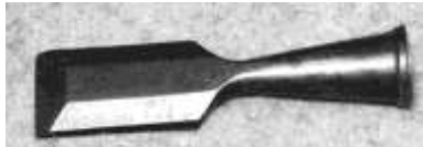
Figure 704. Socket chisel. Steel. Eric Berg. DTM. 102512T15.
