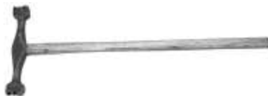
Figure 173. Marking hammer. Cast steel, wood (hickory). Great Northern Paper Company. DTM. 121412T12.
