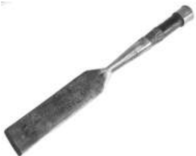
Figure 323. Slick. Forged iron and steel, brass ferrule, wooden handle. Oliver & Daniel Babcock. DTM. 32113T1.
