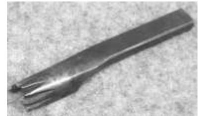
Figure 451. Pinking iron. Cast steel. C. S. Osborne. CLT. 101412LTC2.
