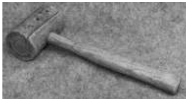
Figure 447. Rawhide mallet. Rawhide, wood (hickory). Garland. CLT. 92812LTC1.
