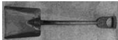
Figure 668. Railroad coal shovel. Cast steel, wood (maple). DTM. 101312T3.
