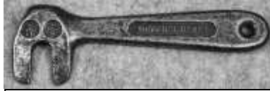
Figure 145. Horseshoe calk wrench. Cast iron. Neverslip. CLT. 7612LTC3.
