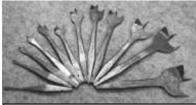
Figure 250. Center bit set. Cast Steel. Various makers. CLT. 63012LTC1.
