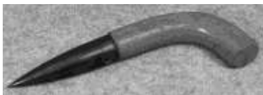
Figure 457. Dibble. Drop-forged steel with red painted wooden handle. DTM. 31212T17.
