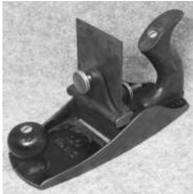
Figure 645. Stanley no. 112 carpenters' scraper plane. Grey cast iron, steel blade, brass nuts, with a wooden tote and handle. DTM. 22211T28.
