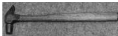
Figure 137. Farriers' clean claw hammer. Cast steel, wood (hickory). Heller Brothers. DTM. 101312T11.
