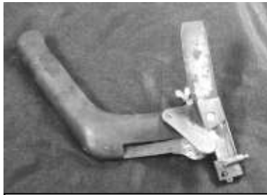
Figure 444. Leather chamfer. Wood, brass, steel. DTM. 111001T35.
