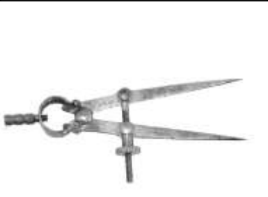
Figure 597. Dividers. Tempered alloy steel. L.S. Starrett. DTM. 111412T5.
