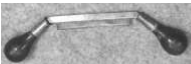
Figure 344. Cabinetmakers' drawknife. Drop-forged steel, wood, painted black. Charles E. Jennings. DTM. 31808SLP17.
