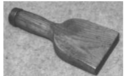
Figure 395. Coopers' bung. Wood, steel ferrules. DTM. 102512T21.
