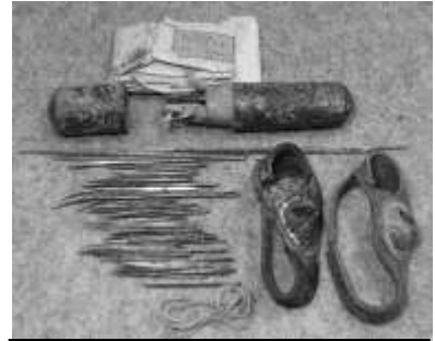
Figure 539. Sailmakers' kit. Cast steel, wood, leather, paper, cotton twine. DTM. 42012T6.
