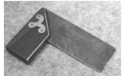
Figure 340. Cabinetmakers' try square. Drop-forged tempered alloy steel, brass, rosewood. DTM. 3312T14.
