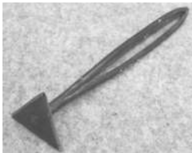
Figure 366. Ship scraper or deck scraper. Forged malleable iron. CLT. 72612LTC1.
