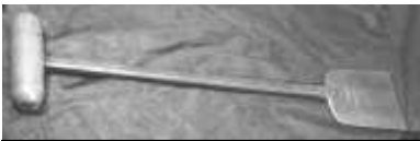
Figure 320. Carpenters' clapboard slick. Forged iron and steel, wood handle. Billings, Augusta. DTM. 52403T3.
