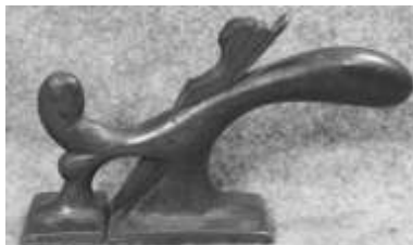
Figure 419. Carriage-makers' plane. Wood with steel blade. DTM. 51703T1.
