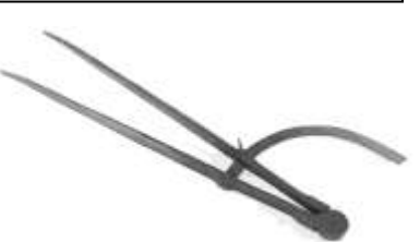
Figure 600. Wing divider. Cast steel. DTM. 31311T9.
