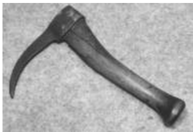
Figure 197. Lumber pick. Low carbon steel. DTM. 93011T6.
