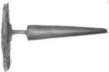
Figure 424. Hub reamer auger. Forged iron, wood. DTM. 72013T3.
