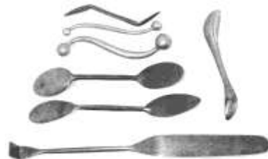
Figure 432. Patternmakers' tools. Cast steel, brass, and bronze. DTM. TCT1004, TCT1301, 62202T9, TCT1006, TCT1007, 121600T3, TCT1003.
