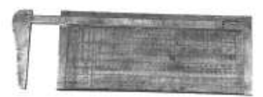
Figure 543. Cordage rule. Boxwood and brass. John A. Roebling. DTM. 42602T2.
