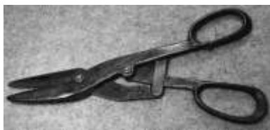
Figure 123. Tinsmiths' levered shears. Drop-forged tempered alloy steel. CLT. 3912LTC1.
