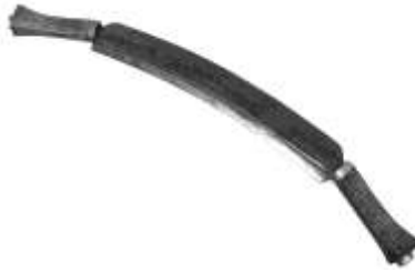
Figure 527. Curriers' fleshing knife. Cast steel, wood (rosewood). Snow & Nealley. DTM. 121412T13.
