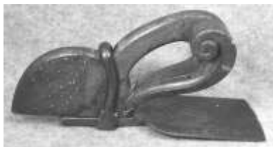
Figure 22. Hand adz. Forged steel, iron, and wood. DTM. 4150T1.
