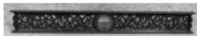
Figure 712. Inclinometer. Drop-forged iron and steel, brass. Davis Level & Tool Co. DTM. 120907T2.
