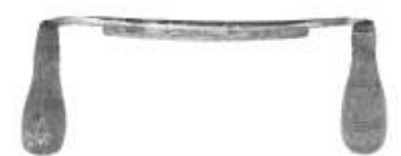
Figure 343. Drawknife. Forged iron and steel with laminated edge, brass, wood (rosewood) handles. J. T. Coffin & Son. DTM. 12812T4.
