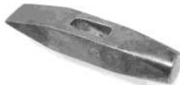
Figure 190. Silversmiths' hammer. Cast steel. DTM. 2713T1.
