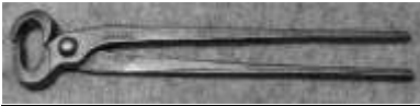
Figure 147. Farriers' hoof parer. Cast iron, cast steel. Champion Tool Co. DTM. 101312T28.
