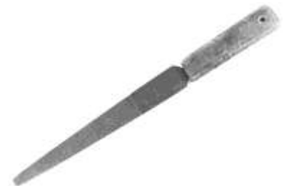
Figure 301. Planemakers' float. Cast steel, wood. DTM. 31212T14.
