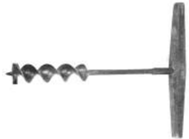
Figure 249. Carpenters' auger. Forged iron and steel, wood handle. C. Drew. DTM. 111002T1.
