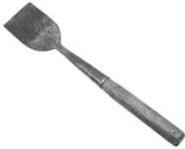
Figure 356. Slick. Forge-welded steel, wood (oak). DTM. 121412T5.
