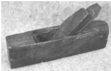
Figure 264. Spar plane, wood (beech), cast steel blade, signed J. R. TOLMAN HANOVER MASS on body and WILLIAM ASH & CO on blade. DTM. 42904T7.
