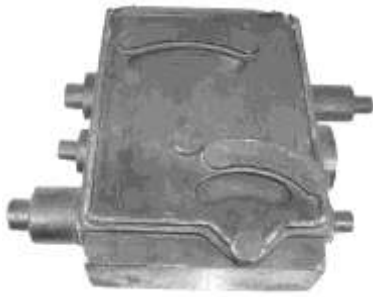
Figure 192. Silver flatware molds. Towles Silversmiths. Cast steel. CLT. 6113LTC1.
