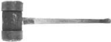
Figure 169. Wooden ringed maul. Wood (oak, hickory), forged iron. DTM. 12713T3.
