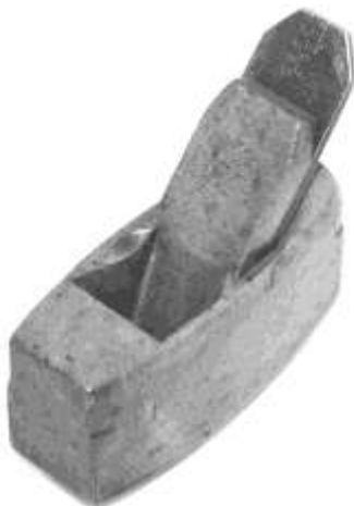
Figure 434. Patternmakers' block plane. Wood (boxwood), cast steel. DTM. 62202T5.
