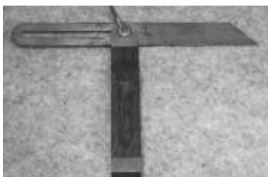
Figure 66. Carpenters' sliding T-bevel. Steel blade, brass trim, and rosewood handle. DTM. 31808SLP19.
