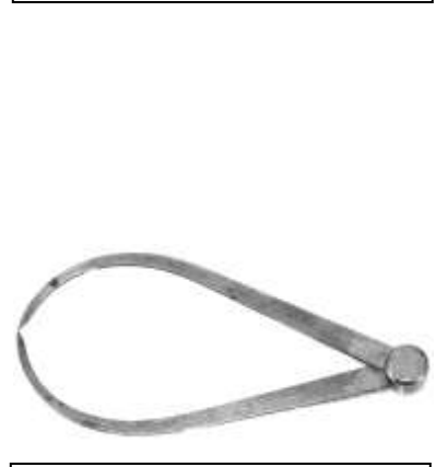
Figure 598. Firm-adjust calipers. Steel. D.E. Lyman. DTM. 102503T2.
