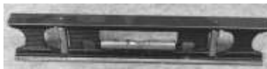
Figure 570. Metallic plumb and level. Grey cast iron, steel, nickel plating, japanned finish. CLT. 52712LTC3.
