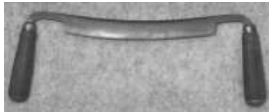
Figure 318. Drawknife. Steel, wooden handles. C. J. Kimball. DTM. 102612T9.
