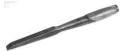
Figure 226. Mortising chisel. Cast steel, wood (beech). J. Russell. DTM. 3213T3.
