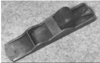
Figure 261. Brass low angle block plane. Cast bronze with cast steel blade. DTM. 22512T4.
