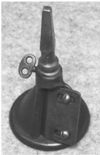
Figure 347. Dowel pointer. Malleable cast iron, steel. DTM. 22311T11.
