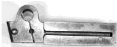
Figure 8. Lathe tool holder. Steel. Signed "WM AVERY & CO FOXBORO, MASS PAT. AUG. 11, 1908." DTM. 21201T12.
