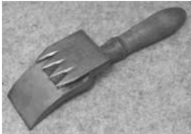
Figure 521. Ice chopper and scoop. Drop-forged steel, wood (rosewood). North Brothers. DTM. 101312T13.
