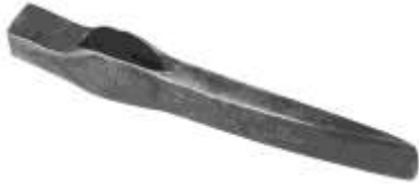
Figure 79. Mortising ax. Cast or forged steel, wood. DTM. 72206T3.
