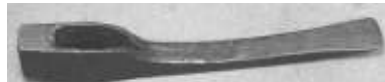
Figure 231. Mortising ax, forge-welded iron and steel. Used for timber framing. DTM. 72206T2.
