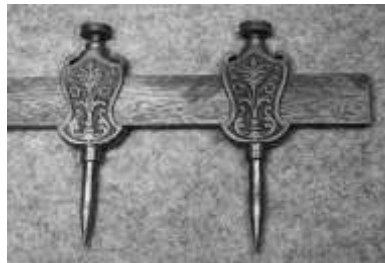
Figure 426. Trammel points. Bronze and oak. DTM. 32708T51.
