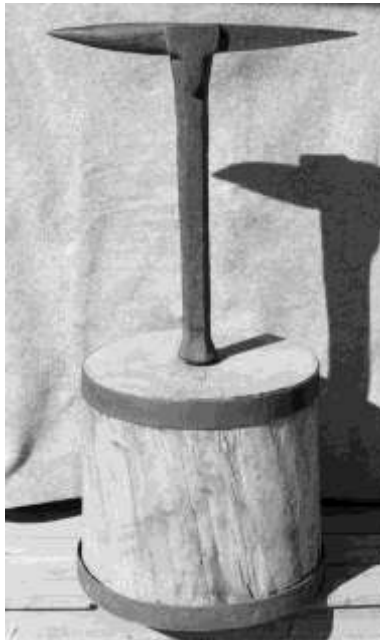
Figure 39. Stump anvil. Forged iron and steel, wood. DTM. 51610T1.
