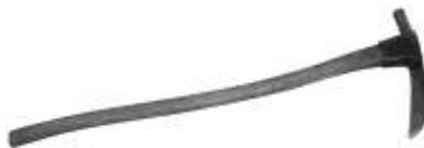
Figure 360. Peen adz. Forged iron and steel, wooden handle. J. Stuart. DTM. 12712T2.
