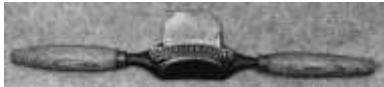
Figure 391. Coopers' drawshave. Cincinnati Tool Co. Cast iron, steel, wood (oak). CLT. 82512LTC1.
