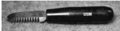
Figure 456. Shoe or saw toothed tack puller. Steel, Bakelite. United Shoe Machine Company. CLT. 52612LTC2.
