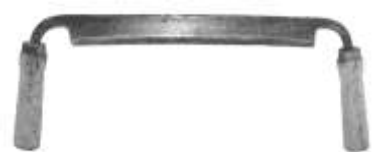
Figure 312. Drawshave. Cast steel, wood (hornbeam). Snow & Nealley. DTM. 121412T1.
