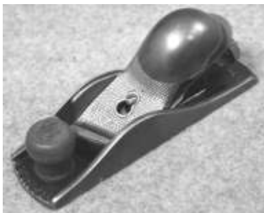
Figure 638. Stanley no. 140 Block plane. Grey cast iron, steel blade, rosewood knobs. CLT. 42812LTC4.
