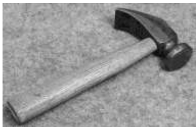
Figure 441. Cobblers' hammer. Drop-forged steel, hickory wood handle. DTM. 32412T4.
