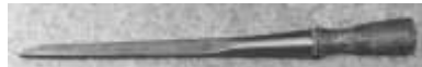
Figure 225. Mortising chisel. Drop-forged iron and cast steel, wood. H.T. Blodget. DTM. 22512T12.
