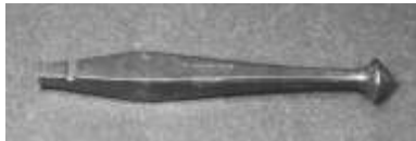
Figure 253. Snail countersink bit. Wood (rosewood), cast bronze, steel cutters. DTM. 81212LTC6.
