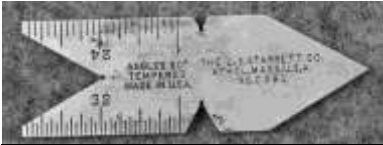
Figure 566. Center gauge. Tempered alloy steel. L.S. Starrett. CLT. 42912LTC17.
