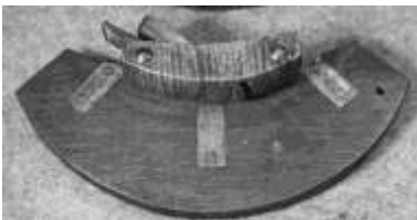
Figure 378. Howel. Wood and steel. DTM. 42801T7.
