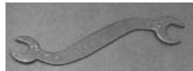
Figure 628. Curved open box wrench. Natural steel. DTM. 8912T3.
