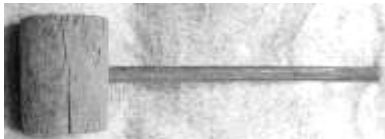
Figure 478. Fence post maul. Wood (oak?). DTM. 102012T1.
