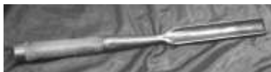
Figure 157. Framing gouge. Cast steel, iron ferrule, hickory handle. J. Gray. DTM. 31212T15.
