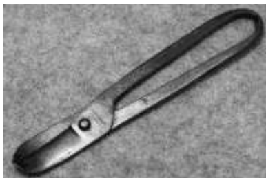
Figure 120. Curved sheet metal snips. Forged steel. DTM. 22411T20.
