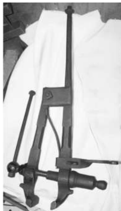
Figure 42. Leg vise. Forged iron and steel. CLT. 12813LTC2.
