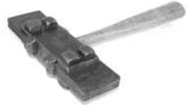
Figure 171. Bush hammer. Cast steel, wood (hickory). CLT. 22813LTC4.
