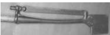
Figure 482. Chisel edge pruning saw. Cast iron, malleable iron, and steel. DTM. 7309T4.
