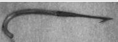
Figure 461. Hay thief. Forged iron, wood handle. DTM. 102904T16.
