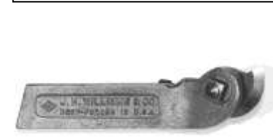
Figure 602. Threading tool holder. Drop-forged steel. J.H. Williams. CLT. 32313LTC7.
