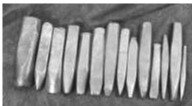
Figure 177. Chasing Stamps, forged steel. Forged steel. W. Jessop & Sons. DTM.
