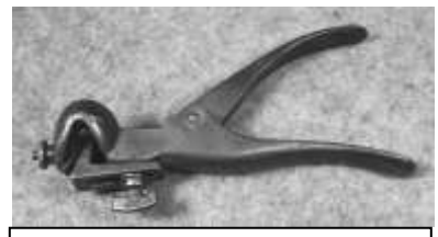
Figure 400. Saw set. Drop-forged iron. CLT. 42912LTC7.
