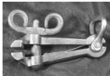
Figure 24. Hand vise, iron and forged steel, signed "P Stubs". Iron and forged steel. Peter S. Stubs. DTM. 62406T7.
