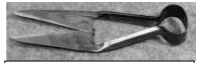
Figure 468. Grass shears. Drop-forged steel. CLT. 6712LTC3.
