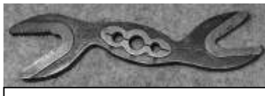
Figure 615. Combination alligator wrench and screw threader. Cast steel. Bonney Vixen. DTM. 101312T18.
