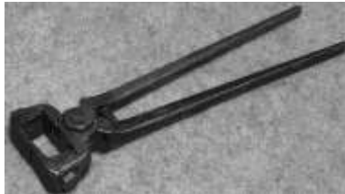
Figure 148. Farriers' end cut nippers. Cast iron, cast steel. Champion DeArment. DTM. 101312T24.
