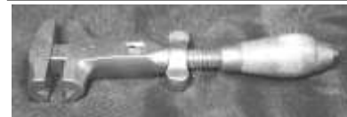
Figure 420. Double jaw buggy wrench. Drop-forged steel, wooden handle. Portland Wrench Co., H.A. Thompson patent. DTM. 041403T1.
