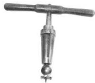
Figure 388. Coopers' bung borer. Forged iron and steel, wood. DTM. 100400T17.
