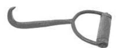
Figure 495. Cargo hook. Malleable iron and steel, wood (rosewood). Snow & Nealley Co. DTM. 121412T3.
