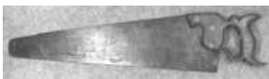
Figure 309. Hand saw. Cast steel, solid brass, wooden handle. B. Biggin & Sons. DTM. 072112T2.
