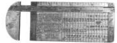
Figure 544. Cordage rule. Boxwood and brass. John A. Roebling. DTM. 82709T1.
