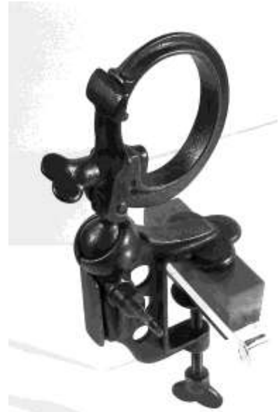
Figure 502. Embroidery hoop clamp. Iron and steel, japanned finish. Courtesy of George Short. 6712LTC1.
