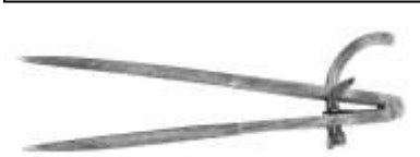
Figure 599. Wing divider. Iron and cast steel. Harrington. DTM. 111412T4.
