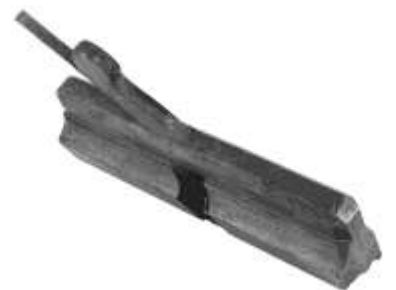
Figure 269. Complex molding plane. Wood (yellow birch), steel blade. John Flynn. DTM. 71504T3.
