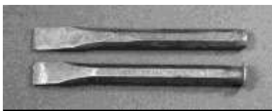
Figure 60. Cold chisels. Silicon manganese alloy steel. DTM. TJD1008.
