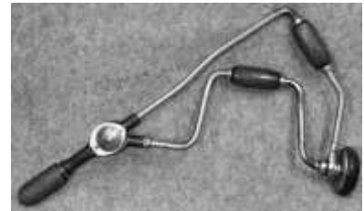
Figure 658. Millers Falls no. 502 corner bit brace. Cast iron, nickel plated finish, wood (cocobolo). CLT. 93012LTC1.
