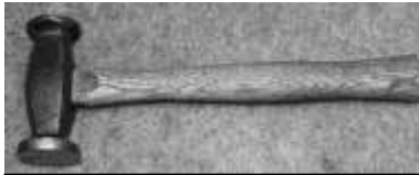
Figure 129. Brass face hammer. Cast steel, wood (hickory), brass. CLT. 10112LTC4.
