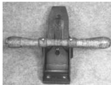
Figure 640. Stanley no. 11 belt-makers' plane. Grey cast iron, wood (beech), cast steel blade, japanned finish. CLT. 6312LTC2.
