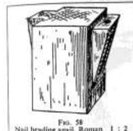
FIG. 58 Nail heading anvil, Roman 1 : 2 Taken from Book of Tools. (From Mr. John Catchings)
