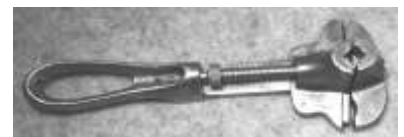
Figure 619. Combination wrench and cutter. Drop-forged steel, nickel plating. CLT. 52712LTC2.
