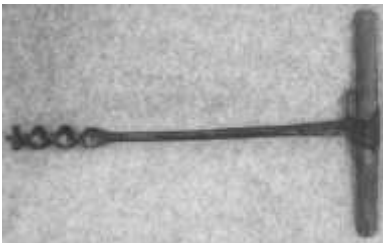
Figure 255. Ring auger. Hand-forged steel, wood. T. Snell. DTM. 72712T1.
