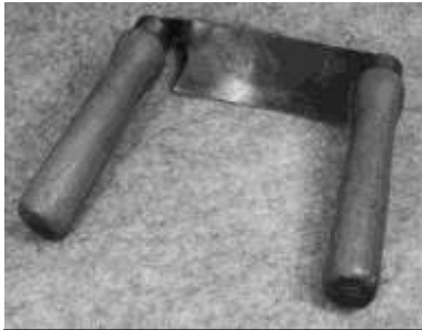
Figure 381. Coopers' hollowing drawknife. Forged steel, wood. Snow & Nealley. DTM. 31212T3.
