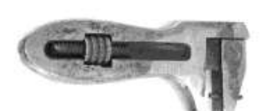
Figure 633. Adjustable wrench. Drop-forged German steel, nickel-plated finish. DTM. 52603T1.
