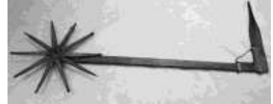
Figure 217. Walking wheel caliper. Wood, brass. LTC. 12812LTC1.
