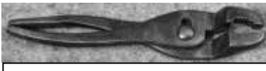
Figure 683. Offset slip joint pliers. Drop-forged tool steel. H.D. Smith & Co. of Plantsville, Connecticut. CLT. 52712LTC4.
