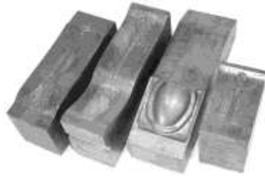
Figure 193. Silver flatware molds. Towles Silversmiths. Cast steel. CLT. 6113LTC1.
