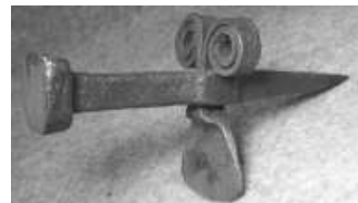
Figure 462. Scythe anvil. Wrought iron with a low carbon steel anvil top. DTM. 111406T3.
