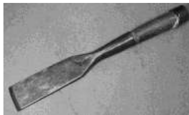
Figure 2. Socket chisel. Forged steel, malleable iron. Signed "J. BRIGGS". DTM. TCC2004.
