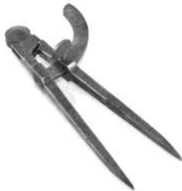
Figure 594. Wing divider. Cast steel. C. Delsten & Sons. DTM. 31908T29.
