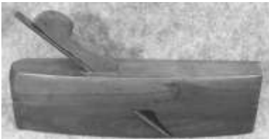
Figure 273. Rabbet plane. Lignum vitae with an oak wedge and a steel blade. DTM. 32802T8.
