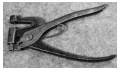
Figure 121. Tinsmiths' hand punch. Drop-forged iron and steel. DTM. 5212LTC2.
