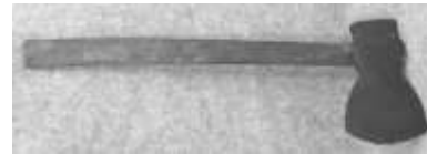
Figure 205. Felling ax. Iron, steel, wood. W. Griffin. DTM. 072112T3.
