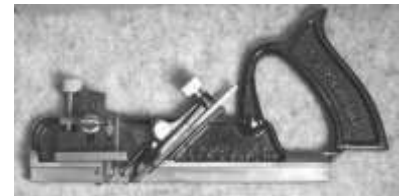
Figure 652. Dado plane. Grey cast iron, japanned finish, steel blade. Stanley. CLT. 7712LTC4.
