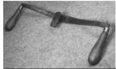
Figure 423. Carriage-makers' body knife. Cast steel, brass ferrules, and wood handles. DTM. 30911T5.
