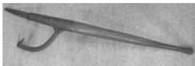
Figure 198. Peavey. Drop-forged iron and steel, wooden handle. Peavey Mfg. Co. DTM. 4106T9.
