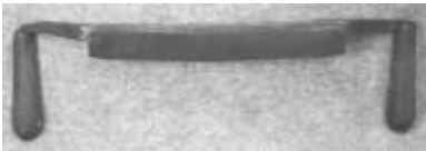
Figure 237. Carpenters' drawknife. Drop-forged steel, wood. DTM. 22512T6.
