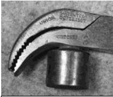
Figure 688. Cobblers' lasting pliers. Drop-forged steel. Whitcher. DTM. 3312T2.
