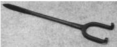
Figure 393. Coopers' flagging iron. Malleable iron and steel. DTM. 102612T12.
