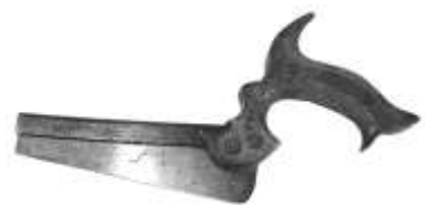
Figure 342. Tapered tenon saw. Cast steel, brass, and wooden handle. R. Groves & Son. DTM. 92911T15.
