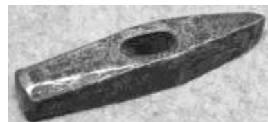
Figure 61. Cold cutter. Steel. Pinel Tool Company. DTM. 072112T4.
