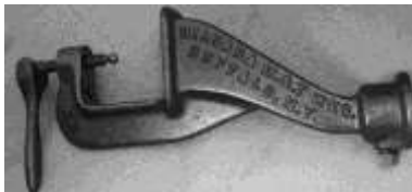
Figure 132. Top: Sheet metal crimper. Drop-forged steel, rosewood grip. CLT. 21812LTC4.
