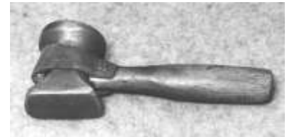
Figure 174. Cobblers' beating out hammer. Steel, wooden handle, leather. DTM. 102512T11.
