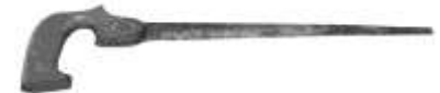
Figure 346. Keyhole saw. Cast steel, brass, wood. William McNiece of Philadelphia. DTM. 121112T5.
