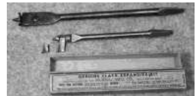
Figure 649. Clark's expansive bit. Cast steel. DTM. 21812T2.
