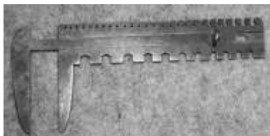
Figure 591. Caliper wire gauge. Cast steel. George Partridge of Darlaston, England. DTM. 42012T4.
