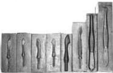
Figure 545. Set of patternmakers' dies for surgical tools. Steel. DTM. 8213T1.
