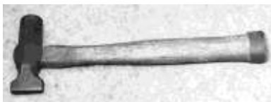
Figure 397. Coopers' bung hammer. Steel, wooden handle. Lang & Jacob. DTM. 102512T3.
