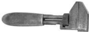
Figure 611. Adjustable nut wrench. Drop-forged steel with cast lead handle. Goodell-Pratt Co. of Greenfield, Massachusetts. DTM. 62202T6.
