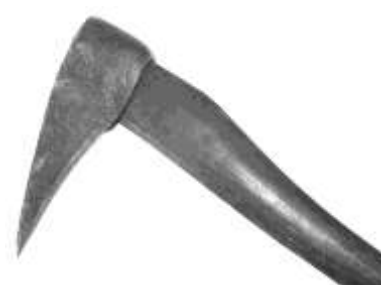
Figure 199. Pickaroon. Forged iron, natural steel, wood. DTM. 102904T5.
