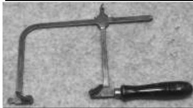
Figure 187. Jewelers' coping saw. German steel, steel blade, hardwood handle. DTM. 22211T24.
