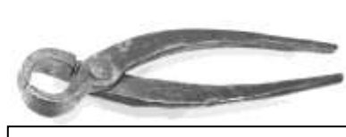
Figure 64. Blacksmiths' end cutters. Forged steel. DTM. 2713T6.
