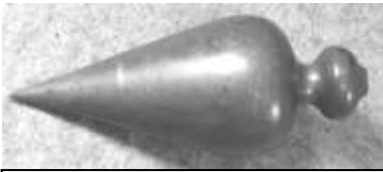
Figure 292. Plumb bob. Brass. C. Drew & Co. CLT. 51312LTC1.
