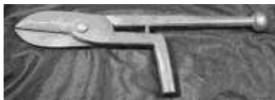
Figure 119. Whitesmiths' bench shears. Forged iron and steel. Peter S. Stubs. DTM. 102100T14.
