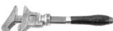
Figure 684. Combination pipe and nut wrench. Cast steel, rosewood, black paint. Bemis & Call. CLT. 2713LTC5.
