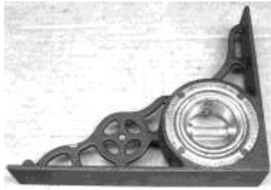
Figure 554. Davis corner level and inclinometer. Cast iron, brass, glass. CRF.
