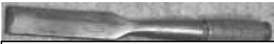
Figure 224. Timber framing socket chisel. Forged iron and cast steel, wood. Underhill Edge Tool Co. DTM. 93011T7.
