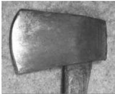
Figure 201. New England pattern ax. Forge-welded iron and cast steel, wood. DTM. 091909T2.
