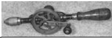
Figure 651. Carpenters' two speed hand drill. Drop-forged malleable iron, steel, and a wooden handle. DTM. 22211T36.
