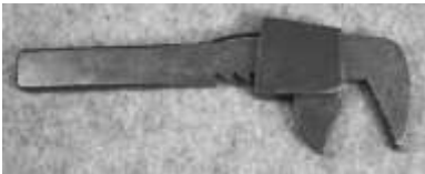
Figure 608. Wedge adjusted wrench. Cast or forged steel. DTM. 101900T6.
