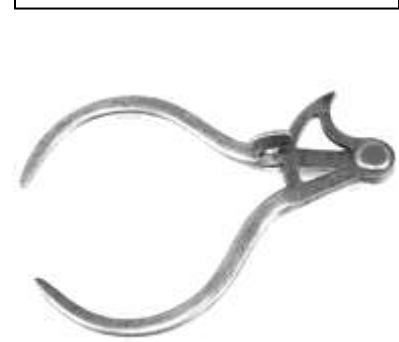
Figure 604. Wing divider. Cast steel. W. Schollhorn. CLT. 32313LTC4.
