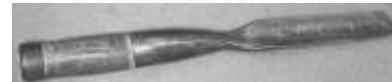
Figure 232. Carpenters' outside bevel gouge. Forged iron, steel, and wood. Horton, New York. DTM. 090109T3.
