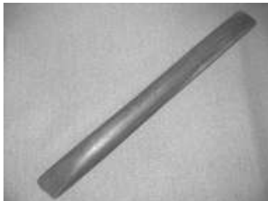
Figure 524. Leather burnisher. Lignum vitae. DTM. 041505T40.
