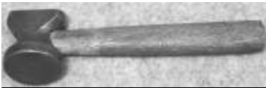
Figure 449. Cobblers' toe or beating out hammer. Cast steel, wood (hickory). United Shoe Machine Company. CLT. 93012LTC5.
