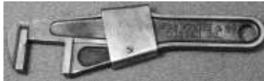
Figure 612. Wedge adjusted nut wrench. Drop-forged steel. Roger Printz & Co. "Fitzall." CLT. 22512LTC2.
