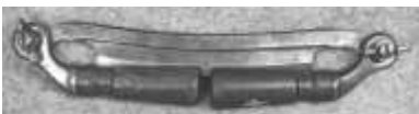
Figure 305. Carpenters' folding drawknife. Forged iron and steel, wooden handle. A.J. Wilkinson. DTM. 52403T4.
