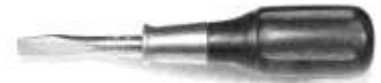
Figure 9. Screwdriver. Drop-forged steel, wood. Signed "Stanley Hurwood Pat April 01 Made in USA." DTM. 111900T11.
