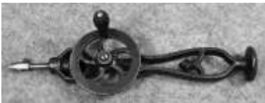
Figure 650. Hammacher & Schlemmer hand drill. Cast iron and steel. CLT. 52612LTC3.
