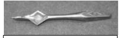
Figure 254. Diamond center gimlet bit. Cast steel. DTM. 8912T8.
