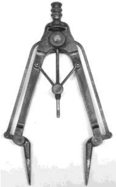
Figure 740. Dividers. Bronze. C. Albert. CRF. Patent #341,714. Ebay, 2001.
