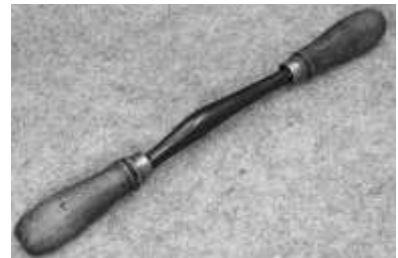
Figure 525. Leather burnisher. Steel, brass ferrules, and wood handles. DTM. 30311T9.
