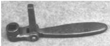
Figure 621. Jointed socket wrench with extension. Drop-forged steel. Abram W. Wheaton. CLT. 7712LTC1.
