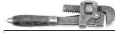
Figure 634. Adjustable pipe wrench. Drop-forged steel, wood (rosewood). F. E. Wells & Son. DTM. 52603T23.
