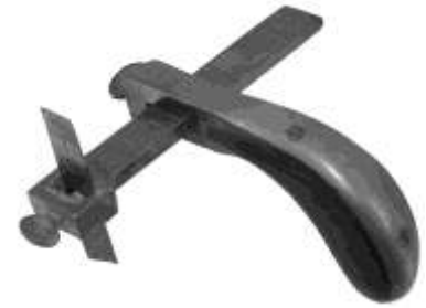
Figure 445. Draw gauge. Drop-forged steel and iron, brass, rosewood. C. S. Osborne & Co. DTM. 102904T20.
