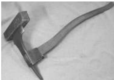
Figure 362. Lipped adz. Formerly in the collection of George DuPrey. Cast steel, hardwood handle (oak?). Plumb. CLT. 21812LTC1.
