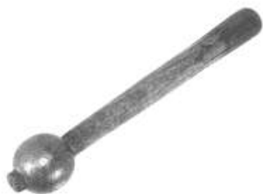
Figure 437. Cobblers' burnisher. Forged iron, wooden handle. DTM. 102904T9.
