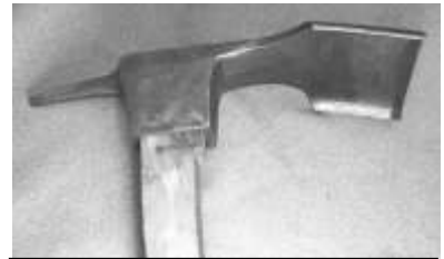
Figure 358. Lipped adz. Formerly in the collection of George DuPrey. Drop-forged cast steel, hardwood handle (oak?). Collins & Co. DTM. 21812T20.
