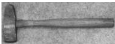
Figure 45. Cross peen hammer. Cast steel, wood (hickory). CLT. 93012LTC4.
