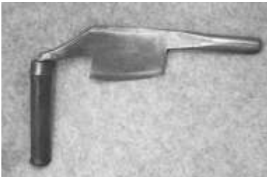
Figure 390. Coopers' chamfer knife. Drop-forged iron and steel, wood. Leonard & Ichabod White. DTM. 41203T6.
