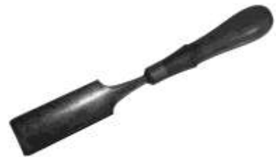
Figure 322. Outside bevel gouge. Cast steel. Holland & Turner. DTM. TCC2002.
