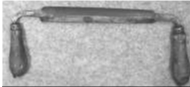
Figure 234. Drawknife. Reforged steel file, hardwood handles, brass ferrules, wood. DTM. 32412T2.
