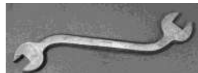
Figure 631. Offset open box wrench. Cast iron. G. Edgcombe. DTM. 8912T2.
