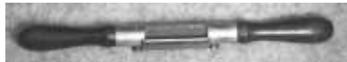
Figure 334. Millers Falls cigar spokeshave. Cast steel, wooden (rosewood) handles. Millers Falls Co. CLT. 7712LTC6.
