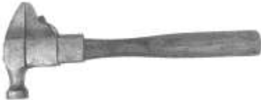
Figure 726. Combination hammer and wrench. C.J. Maggard. CRF. 1902 patent #711,408. eBay, 2012.
