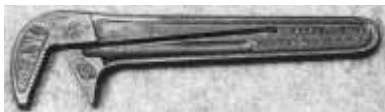
Figure 626. Bryant patent alligator wrench. Drop-forged steel. Shaw Propeller Company, Boston, Massachusetts. CLT. 101212LTC4.
