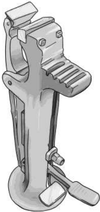
Figure 89. Farrier's Vise. Illustration by Sett Balise, based on vise by B.B. Noyse & Co. of Greenfield, MA.
