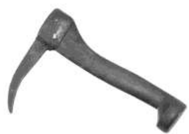
Figure 208. Pickaroon. Forged steel, wood (rosewood). DTM. 121412T17.
