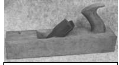
Figure 272. Panel raising plane. Wood (beech), cast steel blade. Abiel F. Walker. DTM. 92001T2.
