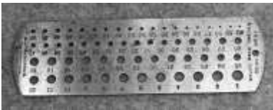
Figure 584. Wire gauge. Steel. Morse Twist Drill & Machine Co. of New Bedford, Massachusetts. DTM. 10910T5.
