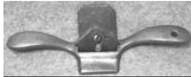
Figure 262. Brass scraper. Cast bronze body, steel blade, malleable iron cap. DTM. 22612T3.
