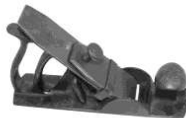
Figure 713. Birmingham plane. Grey cast iron, steel. DTM. TJE1002.
