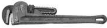
Figure 681. Adjustable pipe wrench. Cast steel, red paint. The Ridge Tool Co., Elyria, Ohio. DTM. 121412T18.
