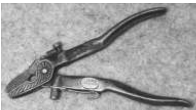
Figure 398. Saw set. Drop-forged steel. Nike of Eskiltuna, Sweden. DTM. 22311T13.
