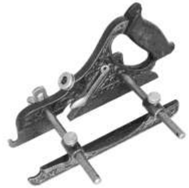
Figure 716. Stanley no. 43 adjustable plow plane. Grey cast iron, brass, wood (rosewood). DTM. 122912LTC1.
