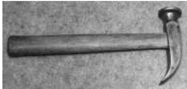
Figure 453. Cobblers' hammer. Steel, wooden handle. Clarkson. DTM. 102512T1.
