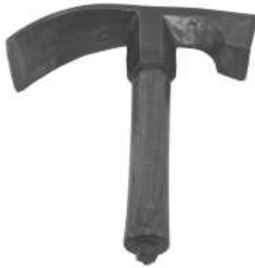
Figure 382. Coopers' adz. Malleable iron and steel with wood handle. DTM. 7602T3.
