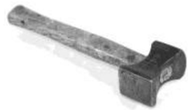
Figure 454. Cobblers' beating out hammer. Cast steel, wood (hickory). CLT. 3213LTC1.
