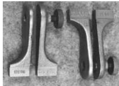
Figure 637. Stair gauge. Drop-forged steel. L.S. Starrett. CLT. 42912LTC6.
