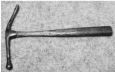
Figure 128. Coppersmiths' bumping hammer. Steel, wooden handle. DTM. 102512T9.
