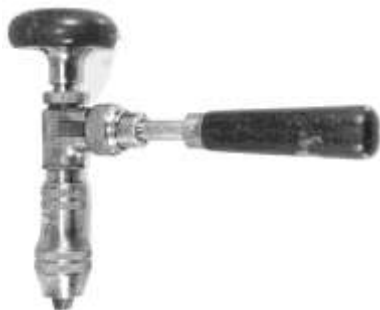
Figure 311. Stanley No. 984 ratcheting corner bit brace. Nickel-plated steel frame with wood (cocobolo) handles. CLT. 81212LTC8.
