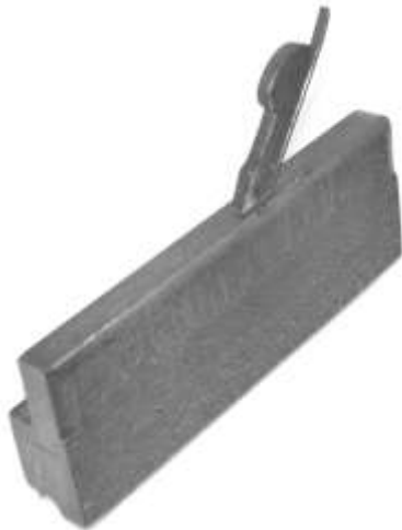
Figure 282. Beading plane. Wood (beech), steel. Joseph Bushell Bridge. CLT. 3713T3.
