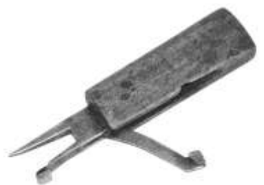
Figure 219. Race knife or timber scribe. Cast or forged steel and wood. DTM. 101400T17.
