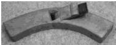
Figure 384. Coopers' sun plane. Wood (bird's eye maple), cast steel blade. Greaves & Co. DTM. 62212T3.
