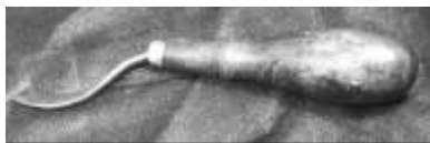
Figure 438. Cobblers' channel gouge. Drop-forged steel, wooden handle, brass ferrule. DTM. 3312T3.
