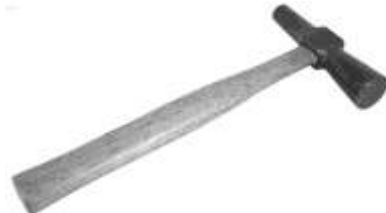
Figure 55. Silversmiths' raising hammer. Cast steel, wood (hickory). DTM. 102512T2.
