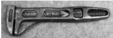
Figure 623. Adjustable tractor nut wrench. Drop-forged grey cast iron. International Harvester Co. CLT. 7612LTC2.
