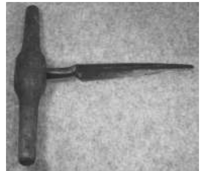
Figure 386. Coopers' tap borer. Forged iron and steel, wood. DTM. TCE1001.
