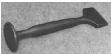
Figure 396. Hoop driver. Cast steel. DTM. 102512T20.
