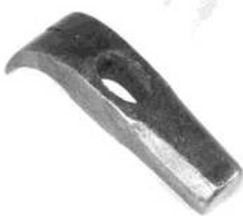
Figure 160. Claw hammer. Forged iron and steel. Warner. DTM. 6703T18.
