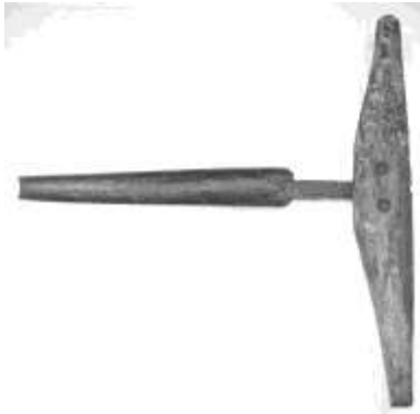
Figure 16. Hub reamer auger. Forged iron, wood. DTM. 72013T2.
