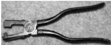
Figure 694. Leather eyelet tool. Drop-forged steel. Eyelet Tool Co., Boston, Massachusetts. DTM. 22612T2.
