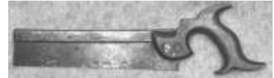
Figure 655. Tenon saw. Cast steel, brass, wood (beech). Unusual “elastic steel” mark. CLT. 8912LTC1.
