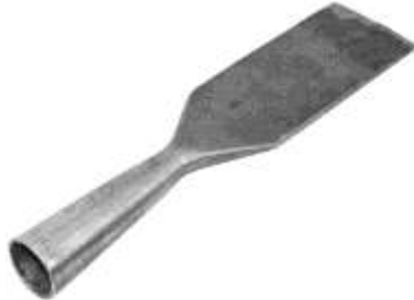
Figure 357. Slick. Forged iron and steel. T.C. Jackson of Bath, Maine. DTM. 121112T1.
