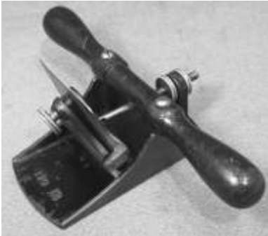
Figure 644. Stanley no. 12 veneer scraper. Grey cast iron, steel blade, brass fittings, wooden handle. DTM. 22211T27.
