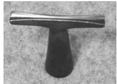
Figure 389. Hoop driver. DTM. Cast steel. 72812T2.
