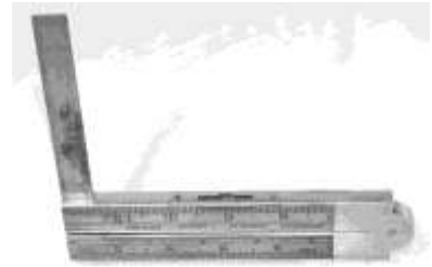
Figure 294. Combination rule. Stephens & Co. CLT. 3213LTC3.
