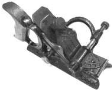
Figure 733. Lee's patent stop chamfer plane. CRF. From a tool picker who bought it for $250 at Brimfield, MA antique sale, 2005.
