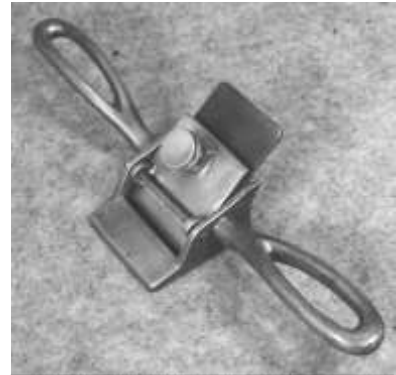
Figure 263. Bronze floor plane. Cast bronze, forged steel blade. CLT. 6912LTC2.
