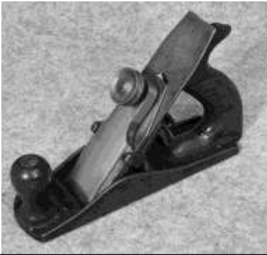
Figure 714. Standard Rule Co. smooth plane. Grey cast iron, cast steel, wood. DTM. TJE4001.
