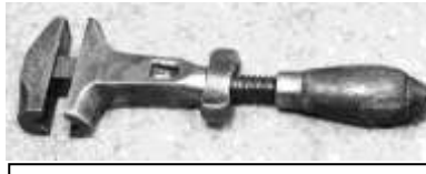
Figure 609. Wagon wrench. Cast steel, rosewood. Diamond Wrench Co., Portland, Maine. CLT. 101212LTC2.
