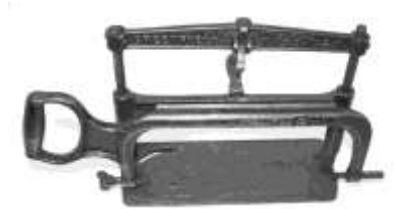
Figure 130. Bench hack saw. Cast iron, wood (rosewood). Goodell Pratt. DTM. TCW1003.
