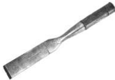
Figure 324. Timber framing chisel. Forged iron and steel, steel ferrule, wooden handle. Dean & Sawyer. DTM. 32113T2.
