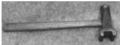
Figure 70. Swage hammer. Cast steel, wood (hickory). CLT. 93012LTC2.
