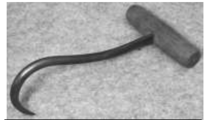
Figure 664. Cargo hook. Drop-forged steel, wood handle. C. Drew, Kingston, Massachusetts. DTM. 22612T1.
