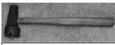
Figure 49. Dolly hammer. Forged iron, wood (hickory). DTM. 101312T5.
