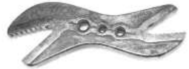
Figure 610. Alligator wrench and pipe threader. Cast steel. DTM. 6703T3.
