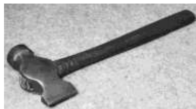
Figure 53. Blacksmiths' straight peen hammer. Steel, wooden handle. DTM. 102512T10.
