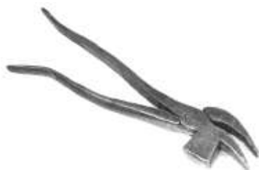
Figure 114. Cobblers' lasting pliers. Forged steel. DTM. 42012T5.
