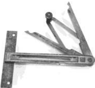
Figure 686. Stanley No. 30 angle divider. Drop-forged steel, nickel finish. CLT. 2713LTC4.
