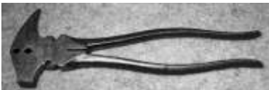
Figure 466. Fencing combination tool. Forged steel. CLT. 42712LTC1.
