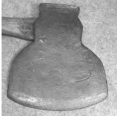
Figure 238. Yankee pattern ax, sometimes called a side ax. Forged iron and natural (?) steel with wooden handle. H. Bragg of Cornville. DTM. 062603T1.
