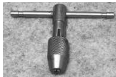
Figure 562. T-handle tap wrench. Drop-forged steel. Dikeman Mfg. Co. of Norwalk, Connecticut. DTM. 22612T9.
