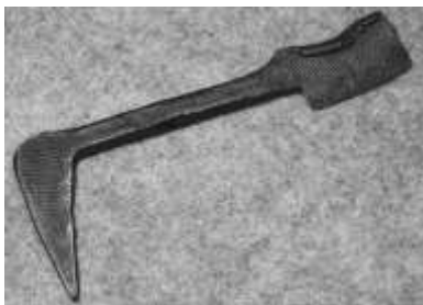
Figure 139. Farriers' toe knife. Forged malleable iron. DTM. 32912T7.
