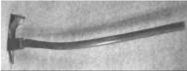
Figure 233. Gutter adz. Forged iron and steel, wood. DTM. 090105T1.
