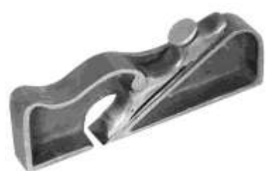
Figure 265. Brass rabbet plane. Cast bronze, steel cutter. CLT. 81212LTC14.
