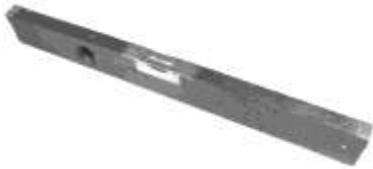
Figure 295. Level. Wood (rosewood), brass, glass. James M. Davidson. DTM. 32313T6.
