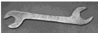
Figure 629. Offset open box wrench. Cast iron. DTM. 8912T9.
