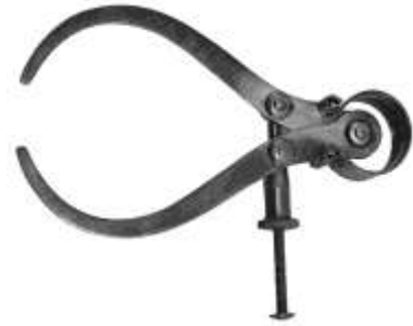
Figure 552. Outside calipers. Forged iron. DTM. 32802T1.
