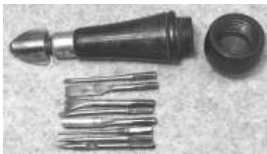
Figure 327. Multi-tool handle. Rosewood handle with drop-forged malleable iron or steel bits. John S. Fray. DTM. 22311T3.
