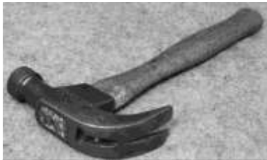
Figure 172. Cheney nailer hammer. Cast steel, wood (hickory). Cheney Hammer Co. CLT. 10112LTC5.
