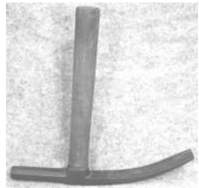
Figure 162. Cobblestone hammer. Forged steel, wood. DTM. 71401T5.
