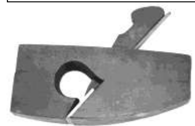
Figure 417. Carriage-makers' plane. Wood (maple), cast steel. CLT. 122712LTC3.
