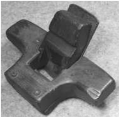
Figure 375. Coopers' down shave. Wood with a forged or cast steel blade. Kenyon, Sheffield. DTM. TCJ1001.
