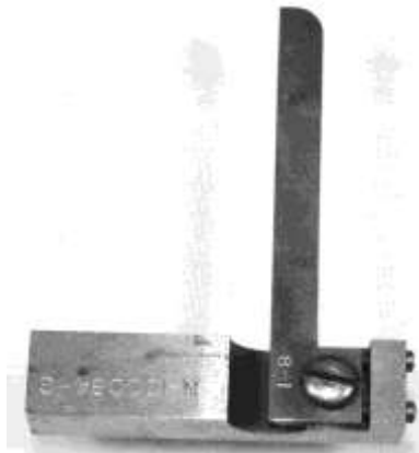
Figure 556. Precision square. Tool steel. Taft & Pierce Mfg. Co. DTM. 81713T14.
