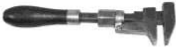
Figure 605. Center adjusted nut wrench. Drop-forged iron, wood (rosewood). Solymon Merrick. DTM. 62406T6.
