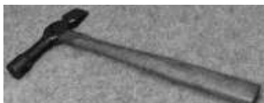
Figure 52. Long reach cross peen hammer. Cast steel, wood (hickory). DTM. 101312T8.
