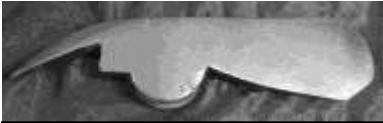
Figure 484. Ice ax. Iron and weld steel. Dernell & Co. of Athens, New York. DTM. 040904T4.
