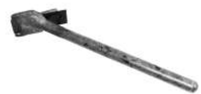
Figure 367. Ship carpenters' scraper. Forged iron, steel, wood. DTM. 71401T9.
