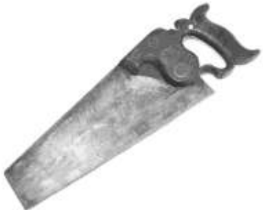
Figure 410. Hand saw. Saw steel, wood (rosewood), brass. T. Tillotson. DTM. TCW1003.
