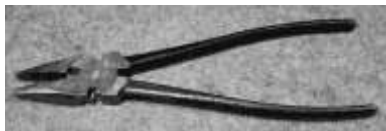
Figure 670. Button patent wire pliers. Drop-forged steel. CLT. 42912LTC11.
