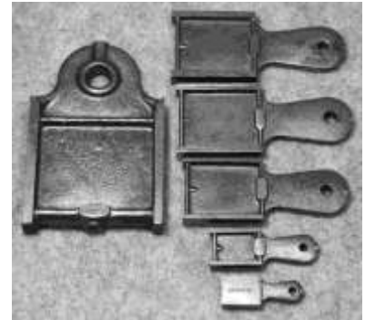
Figure 583. Go nogo inspection gauges. Drop-forged steel, japanned finish. Brown & Sharpe. DTM. 71912LTC1.
