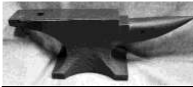
Figure 37. English pattern blacksmiths' anvil. Cast steel. CLT. 22512LTC3.
