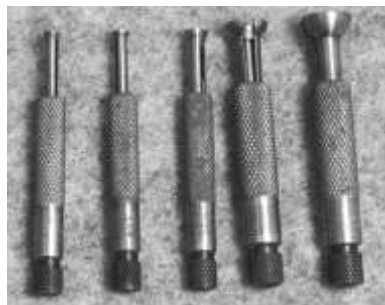
Figure 561. Small hole gauges. Drop-forged tempered alloy steel, vinyl pouch. L.S. Starrett. CLT. 22512LTC7.
