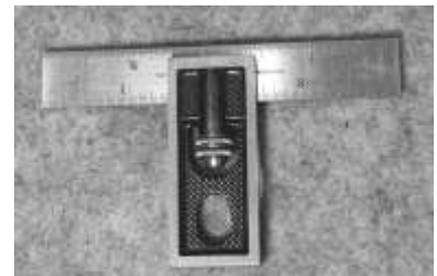
Figure 571. Starrett No. 13 Double Square. Tool steel. CLT. 8512T1.
