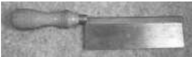
Figure 338. Cabinetmakers' dovetail saw. Cast steel, brass fuller, wooden (beech) handle. William Marples. CLT. 7712LTC7.
