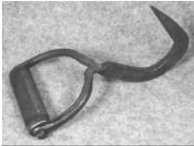
Figure 200. Pulp hook. Drop-forged iron and steel, wood (rosewood). Snow & Nealley. DTM. 31908T39.
