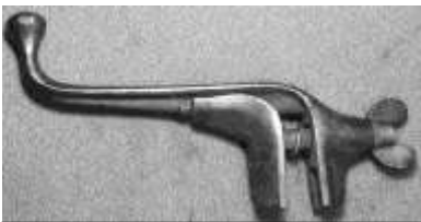
Figure 418. Wagon wrench. Drop-forged steel, brass spring. Reed & Co. of Higgauum, Connecticut. DTM. 21912T1.
