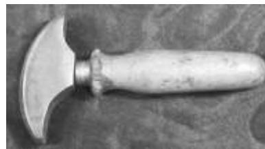
Figure 439. Cobblers' corrugated burnisher. Steel, brass ferrule, wood (beech). DTM. TCH1005.
