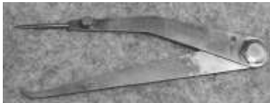
Figure 572. Firm joint hermaphrodite calipers. Tool steel. L.S. Starrett. CLT. 62112LTC1.
