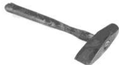
Figure 54. Cold cut hammer. Cast steel, wood (hickory). CLT. 12813LTC1.
