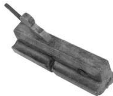
Figure 20. Complex molding plane. Wood, forged steel blade. Robert Wooding. DTM. 50402T1.
